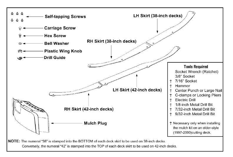
**NOTE:** Due to the fact that OEM-190-116 mulch kit is designed for use on both 38-inch cutting decks and 42-inch cutting decks, not all of the contents of the carton will be used for your tractor's deck application.
